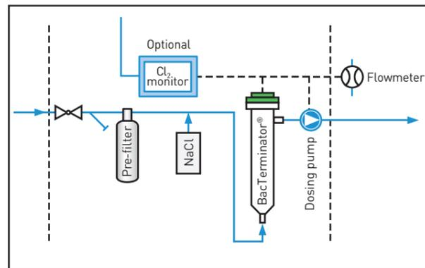
Fig. 2: Process in BacTerminator® Safe
